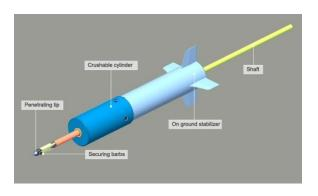
The on-the-ground test harpoon is about 60cm in total length. A space harpoon would not need the winged stabilizer
